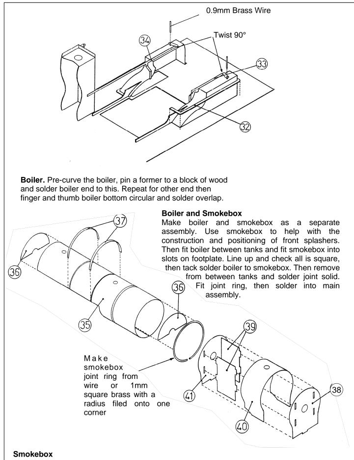
Firmly fix with drawing pins the smokebox front to a block of wood and roughly pre-form the smokebox wrapper using an off cut of pipe and drill shanks etc. Position the wrapper to the centre of the smokebox front top (note etched centre marks). Starting from the top work your way round, soldering to the front and using this as a former. Solder spacers in place, then solder smokebox rear to wrapper.
