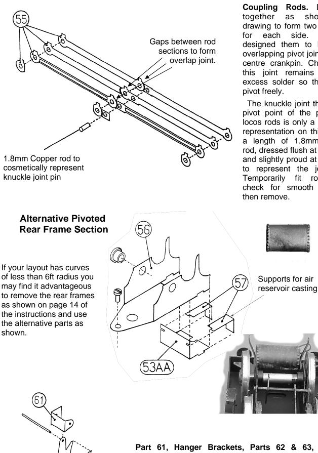
Part 61, Hanger Brackets, Parts 62 & 63, Brake Blocks and Hangers. Fit lengths of 0.9mm brass wire
