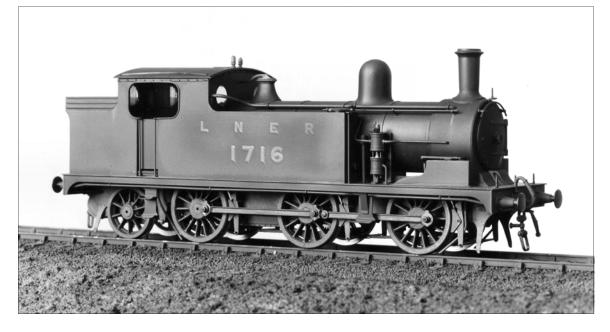
**Prototype.** This class of 20 locomotives were built from 1902. Although mainly intended for mineral and freight train working all of the class were built with Westinghouse brakes. They proved useful on passenger trains and lasted until 1962.
