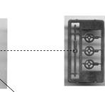
Remove regulator from etch and bend to form handles at ends
