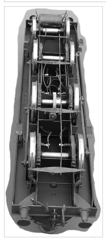
Fit spring castings, these are a standard casting and may need a slight modification to the rear web when fitting.
